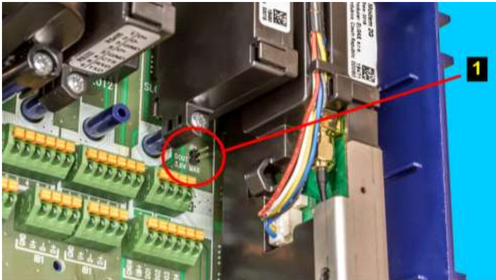
Fig. 58 Placing JP1 Jumper on I/O Board
